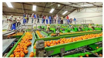
Groep 91's packhouse has an intake capacity of around 500 tonnes per day, using a 10-lane Greefa SmartSort optical grader.
